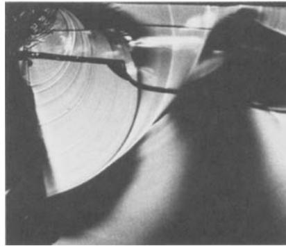
Fig. 2. Half-side view and half-schematic of median/radial crack system in soda-lime glass. Micrograph shows fracture surface of specimens broken at indentation sites; crack-arrest markings are introduced to provide record of crack evolution. Note failure origin at surface trace of half-penny.
